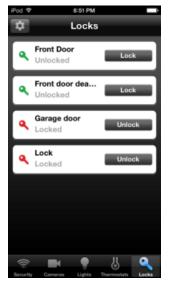
The Door Locks screen shows all the door locks installed at your site, and the current state of each (locked or unlocked). The icon to the left of the name also indicates the state. You can use this screen to remotely lock or unlock any door. Simply tap Lock or Unlock to change the setting of any door on the list.
